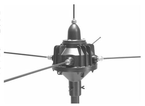
The cable connectors are fitted to the bottom side of the antenna head's bottom flange. It is protected against the environment by a trumpet shaped mounting support (the funnel) which is mounted to the bottom flange of the antenna head. The opposite end of the funnel fits the size of 2" supporting pipes.
